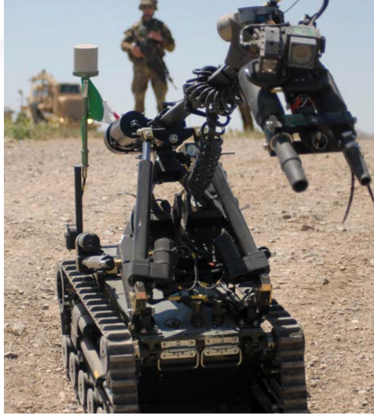
Safer route clearance: robots counter improvised explosive devices (IEDs).
